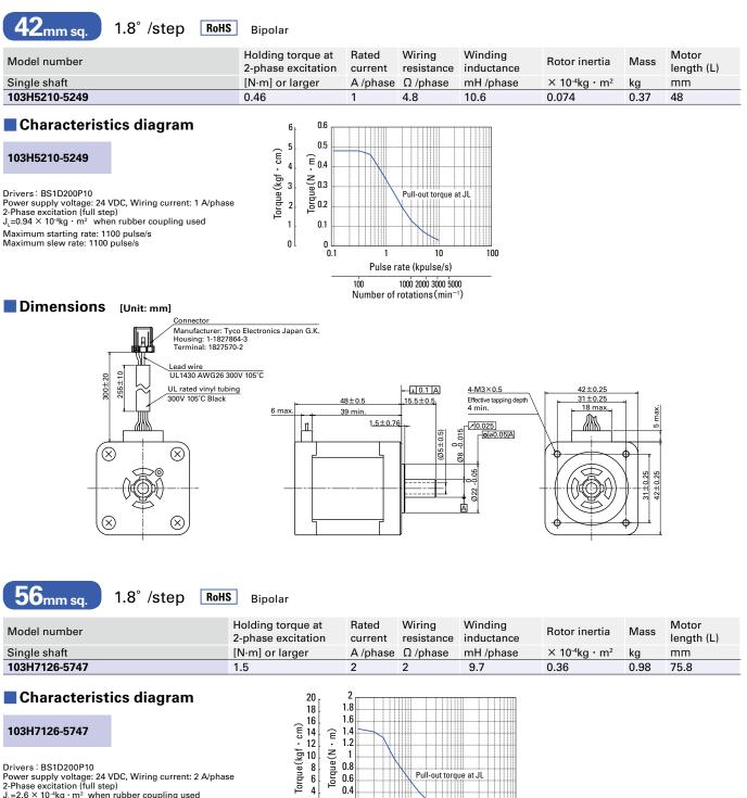
Drivers : BS1D200P10 Power's DSTD200F10 Power supply voltage: 24 VDC, Wiring current: 2 A/phase 2-Phase excitation (full step)  $J_1$ =2.6 × 10<sup>-4</sup>kg · m<sup>2</sup> when rubber coupling used Maximum starting rate: 750 pulse/s Maximum slew rate: 750 pulse/s
