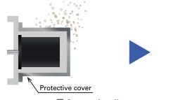
Conventionally Protective cover was necessary to protect the motor against fine particles such as powders.
